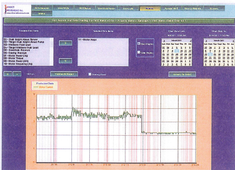
Figure 5. Motor amps/parted rods.
