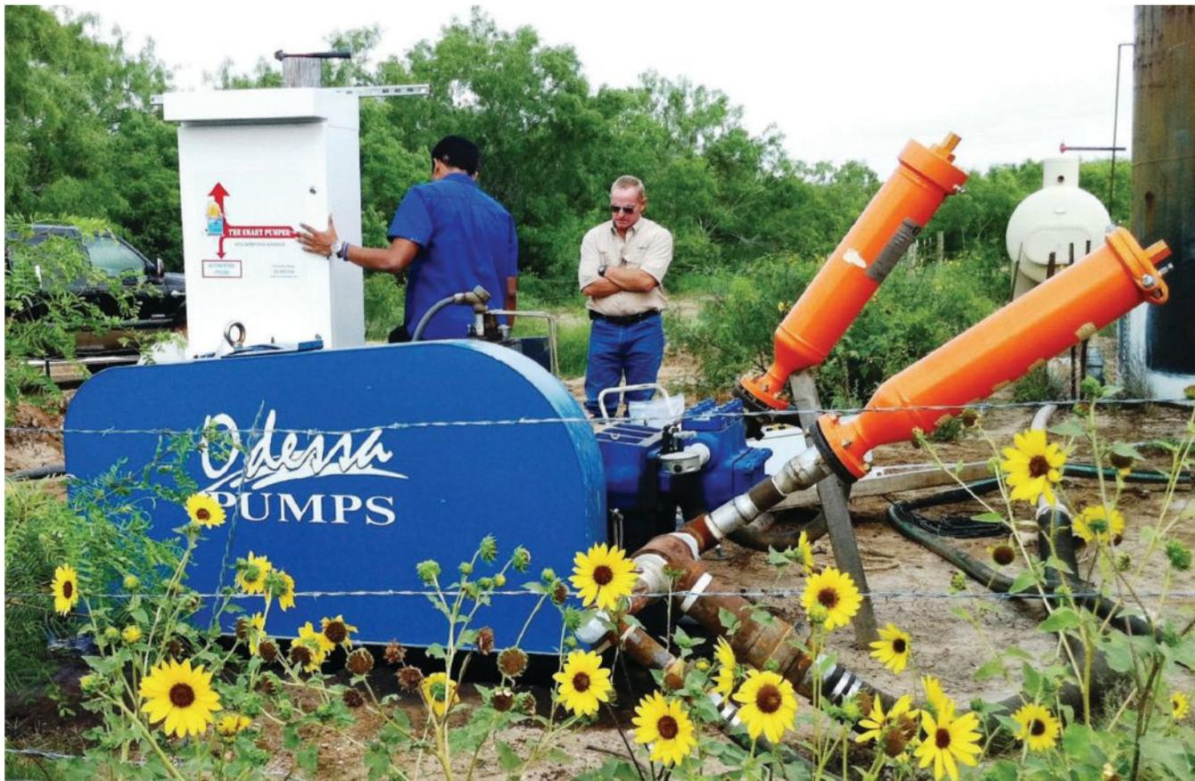
Inside the protective white box is a pump monitoring and control system called the Smart Pumper, installed in the Eagle Ford Shale. It uses fluid level data in a well to maximize production, and limit the risk of pump damage. *Photo courtesy of Direct DriveHead.*
